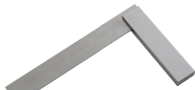
Engineers square Used to scribe 90° lines in metal
